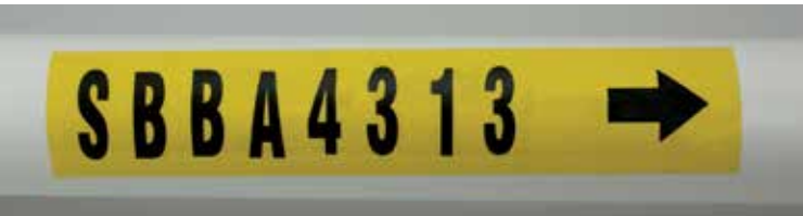
Step 3: Apply characters onto pipe marker.
