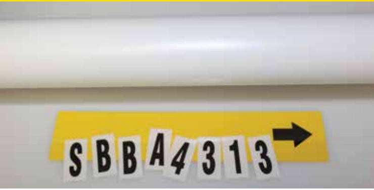
Step 1: Set out blank pipe marker and characters.
